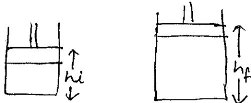
$$\begin{aligned} |\text{Work}| &= \text{Force} \times \text{distance} \\ &= F \times \Delta h \\ &= (P \times A) \times \Delta h \\ &= P \times \Delta V \end{aligned}$$
