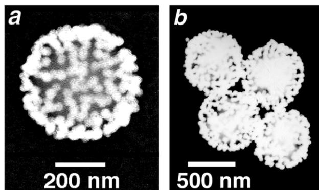
Fig. 1 TEM images (Philips EM-400, 100 kV) of Au/SiO<sub>2</sub> superparticle ensembles. Diameters (in nm): (a) 30/430; (b) 60/550.
