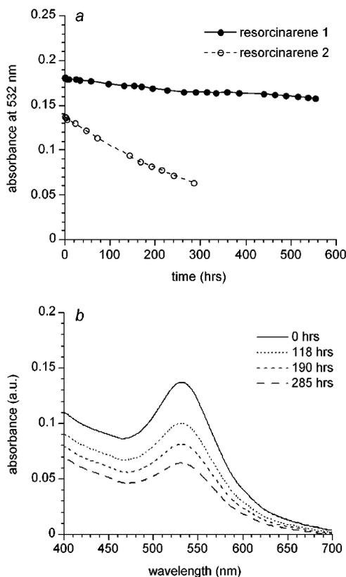
**Figure 3.** (a) Dispersion stability of 19-nm gold particles encapsulated by **1** (circles, filled) or **2** (circles, open) in toluene at 25 °C, monitored by their surface plasmon maxima of 532 nm. (b) Optical extinction spectra of 19-nm gold particles stabilized by **2** over time.
