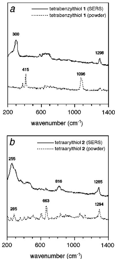
**Figure 7.** Surface-enhanced and powder Raman spectra of **1** and **2**. Spectra were acquired using a micro-Raman spectrometer operating at 785 nm with a 40 $\times$  objective lens (NA = 0.75), an input power of 10 mW at the sample, and an exposure time of 30 s. (a) Tetrabenzylthiol **1** adsorbed onto 40-nm Au particles (—) and in powder form (---); (b) tetraarylthiol **2** adsorbed onto 40-nm Au particles (—) and in powder form (---). Spectra have been shifted for clarity of presentation.
