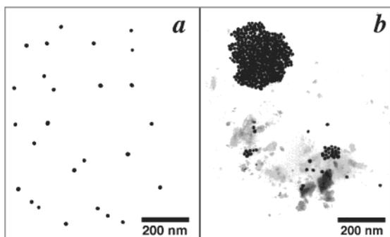
**Figure 5.** Transmission electron micrographs (Philips EM-400, 80 keV) of 19-nm colloidal gold particles stabilized by **1** in the absence (a) and presence (b) of propanethiol. Nanoparticles were dispersed in toluene, aged for 6 weeks, and then dropped onto Formvar-coated Cu grids (300 mesh) and dried by slow evaporation in air. Organic deposits are evident in the propanethiol-treated sample.
