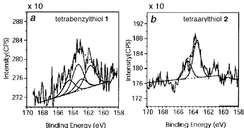
**Figure 8.** X-ray photoelectron spectra of the sulfur 2p regions of **1** (a) and **2** (b) adsorbed on Au(111) surfaces. Each S 2p peak was fitted as two linked components,  $2p_{1/2}$  and  $2p_{3/2}$ . Peak areas of the  $2p_{1/2}$  component were set at half the peak area of the  $2p_{3/2}$  component with a fixed peak separation of 1.2 eV. Dashed lines represent the baseline and total curve fits.
