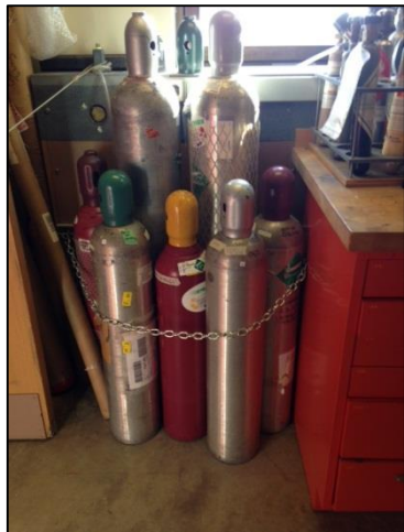
Figure 5.3 – Not In-Use Cylinders
