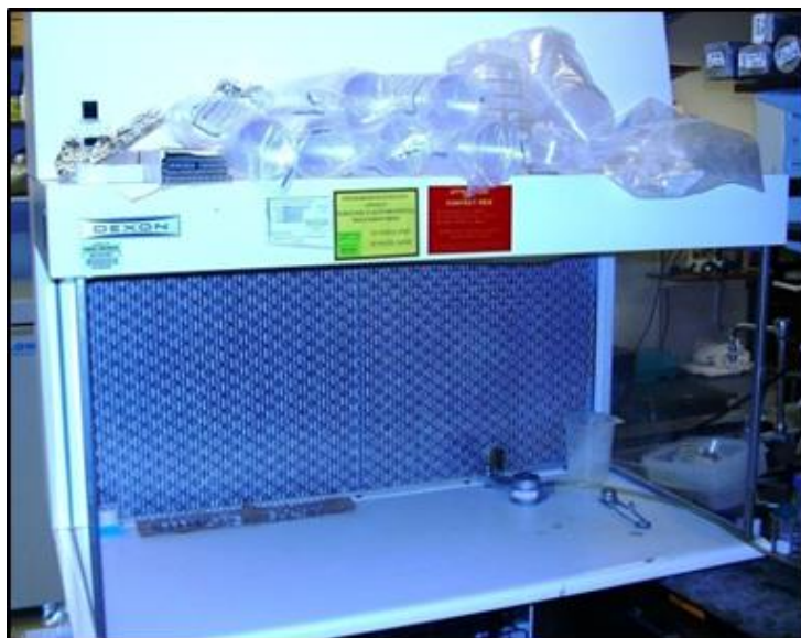
Figure 4.4 – Laminar Flow Clean Bench
