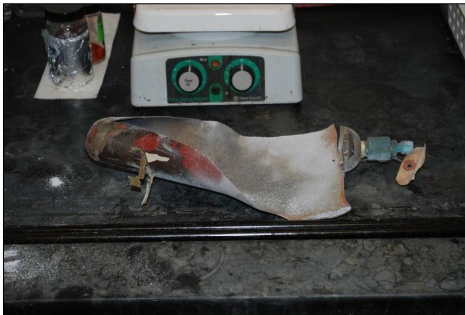
Figure 5.8 – HF Cylinder Incident at Purdue University in 2011
