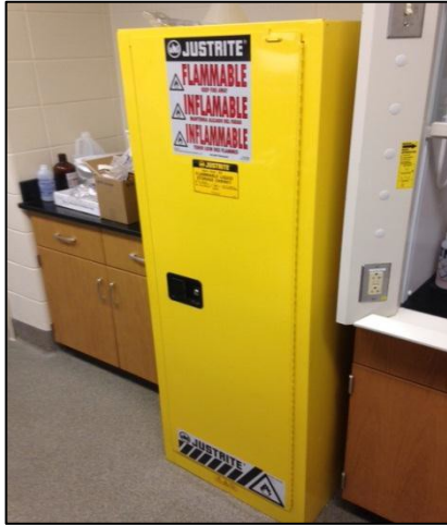
Figure 5.1 – Flammable Storage Cabinet
