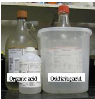
Fig.1- Demonstration of proper use of secondary containment with Organic and Oxidizing acids
