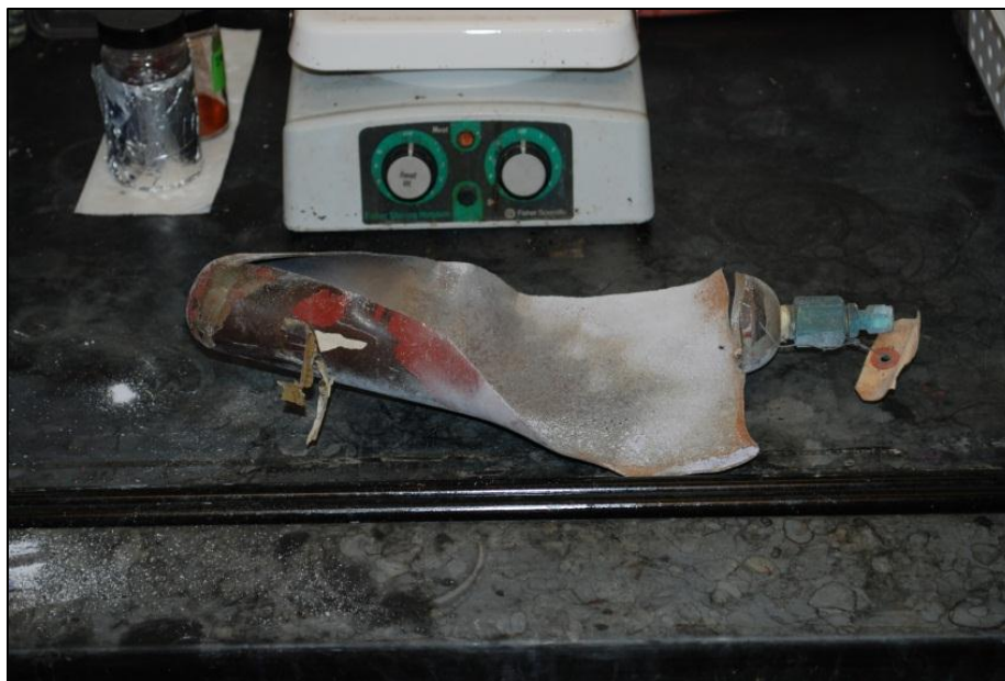
Figure 5.8 – HF Cylinder Incident at Purdue University in 2011
