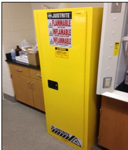
Figure 5.1 – Flammable Storage Cabinet
