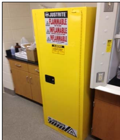
Figure 5.1 – Flammable Storage Cabinet
