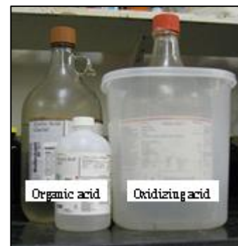
Demonstration of proper use of secondary containment with Organic and Oxidizing acids
