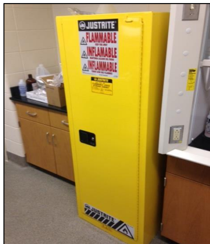
Figure 5.1 – Flammable Storage Cabinet
