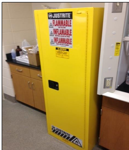
Figure 5.1 – Flammable Storage Cabinet
