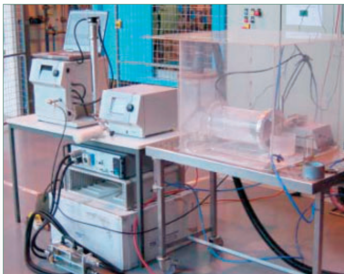
Figure 2 Powder containment chamber used to evaluate the DMA and CPC system supplied by TSI
