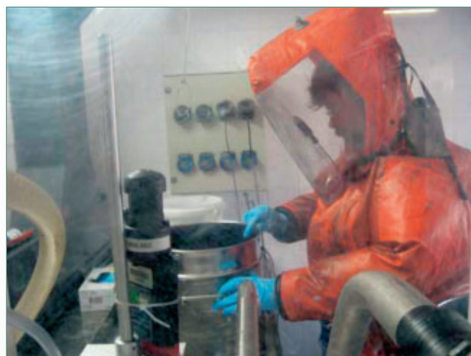
Figure 6 Operator in a secured handling room for nanomaterials
