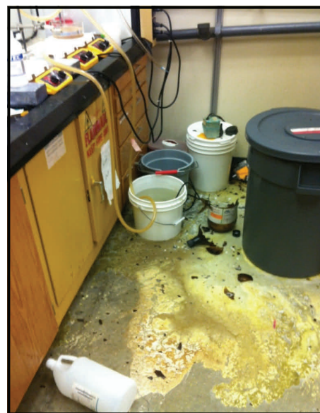
Fig. 2 Purdue, amber glass bottle explosion on the floor.
