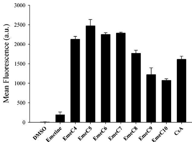
FIGURE 3: Flow cytometry data for MCF-7/DX1 cells treated with R123 (0.5 μg/mL), DMSO, emetine, each of the bivalent emetine agents with hydrophobic tethers, and cyclosporin A (CsA) (10 μM each).
