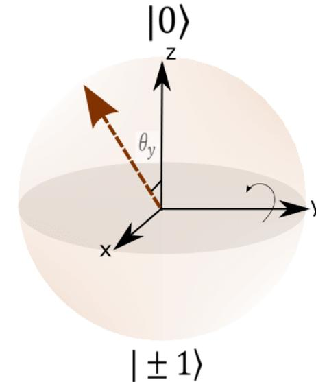
Fig. 11b: Bloch sphere illustration showing the rotation  $\theta$  around y
