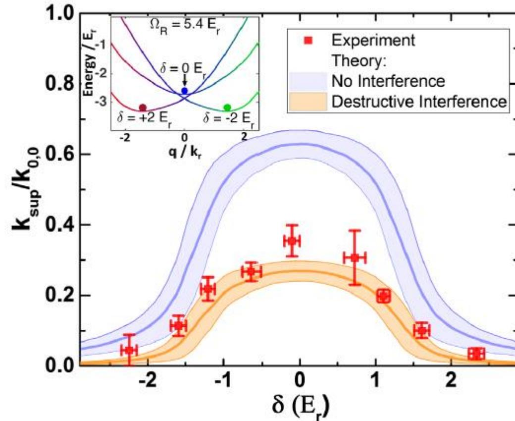
Fig. 9a: Normalized photo-association rate  $k_{\text{sup}}/k_{0,0}$  as a function of  $\delta_r/E_r$  at  $\Omega_r = 5.4 E_r$  (Blasing et. al. , PRL 2018)
