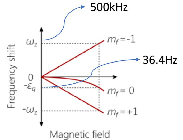
Fig. 6: Schematic representation of Zeeman splitting under bias magnetic field
