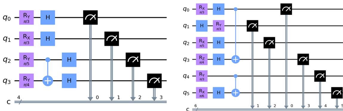
Fig. 2 Sample 4-qubit (left) and 6-qubit (right) quantum circuits for which the quantum states are reconstructed using the proposed approach based on maximal entropy formalism.
