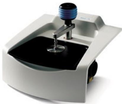
Solid and liquid (see restrictions below) samples usually can be measured without further preparation by putting them directly on the ATR crystal. The 6700 system can be configured to hold liquid and gas cells. **Most liquids (corrosive, poisonous, BSL-II samples, most solvents) must be put in a liquid cell.** Ethanol, methanol, iso-propanol and hexane can be put directly on the ATR crystal. Please contact RIC staff if you don't know if your liquid sample should be put in a liquid cell.
