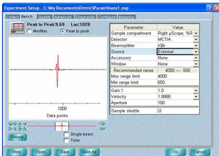
This screen shows the real-time interferogram signal and allows the user to do some spectrometer configuration setup. Assuming you have a sample (which could also be just the air in the compartment) in the sample chamber and that the MCT detector is cooled with liquid nitrogen, you should see a signal like the one shown above.
