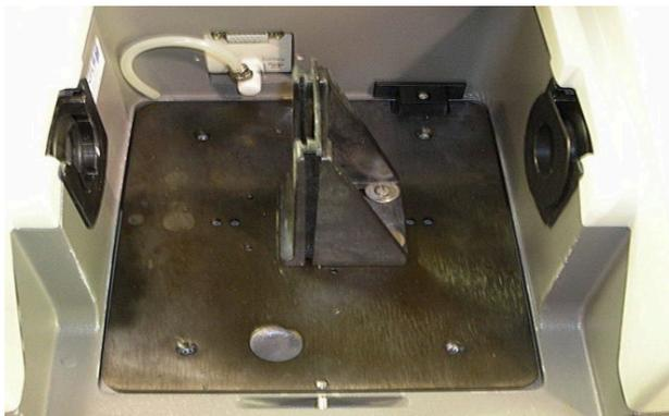
As a rule of thumb, I suggest purging for 1 minute every time you open the sample chamber to change samples. This will give you pretty equal conditions for every background and sample data collection. At the start of your experiment and when the chamber is open for
