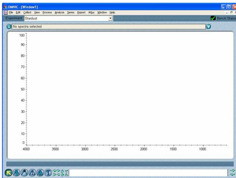
The green check mark on the bench status shows that the spectrometer is ready to go. To check the signal strength and set the spectrometer parameters, go to the Collect Menu, and choose Experiment Setup.
