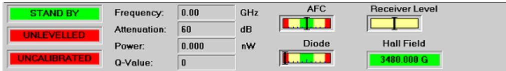
8. Set attenuation to 50dB and use the right/left arrow buttons of the Bias slider to center the Diode Current meter (200  $\mu$ A) in the Instrument Monitor Window
