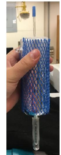
Fluorimeter equipped with Dewar for 77 K measurements
