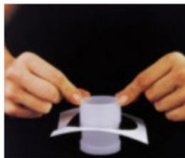
Place the cup or small mass sample holder with the foil down on a clean surface and fill it with your powder or liquid, or place a flat side of the solid onto the foil as close to the center of the cup as possible.
