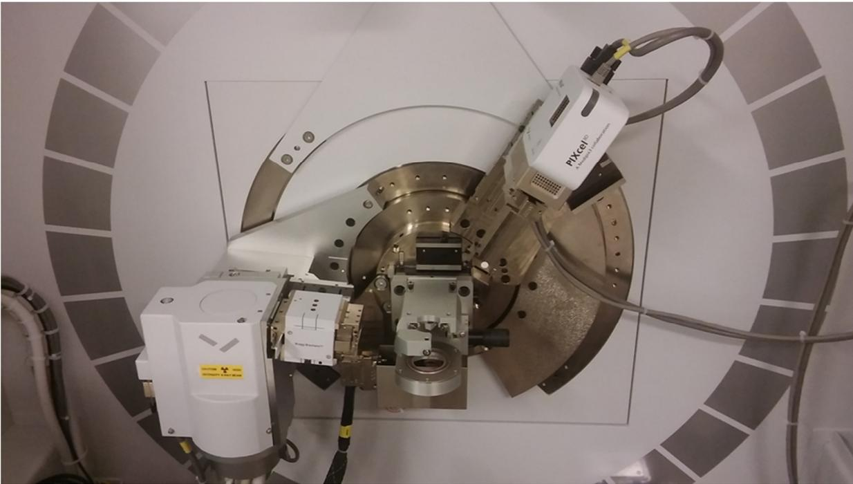
On the Empyrean control PC, check if the “Data Collector” software is running. Start it if necessary. Login in is “user-1”, password is “galaxy”. Once Data Collector is running, go to “Instrument”, then “Connect”. Wait for the software to finish establishing communication with the instrument. When prompted, select the stage that is installed.
