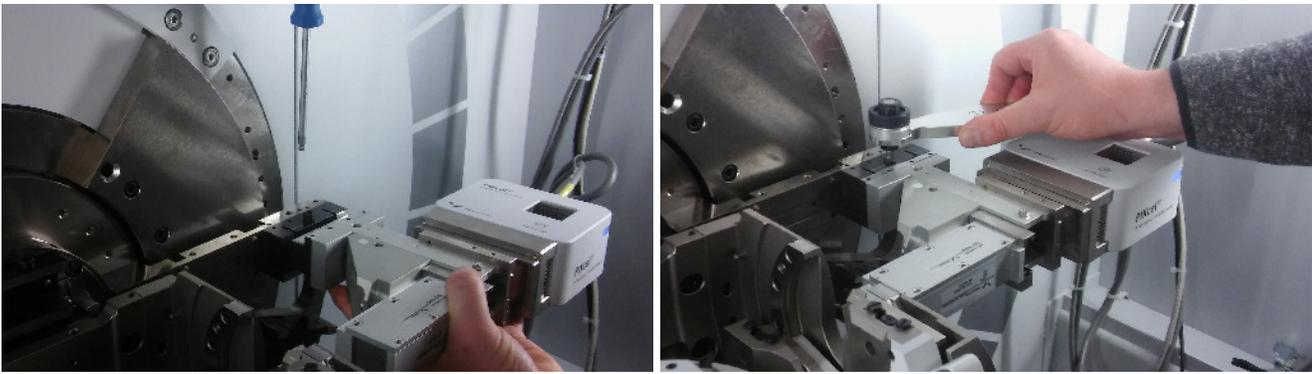
Press the “next” button in Data Collector and wait for the positioning of the instrument to finish.
