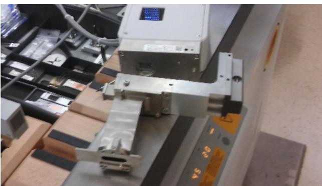
Take off the FASS holder and carefully place it in a save place inside the cabinet.
