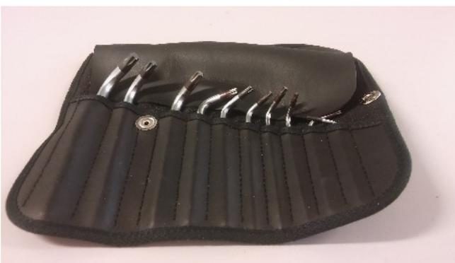
The detector is mounted to the FASS holder with two hex mounting screws and one pin. Loosen the screws completely. Use the T20 hex Allen wrench from the black pouch inside the cabinet for this. The screws will remain with the FASS holder.
