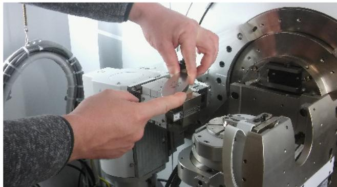
The detector cannot be remounted right away. It first has to be taken off the FASS mount and affixed to the PCC mount instead.
