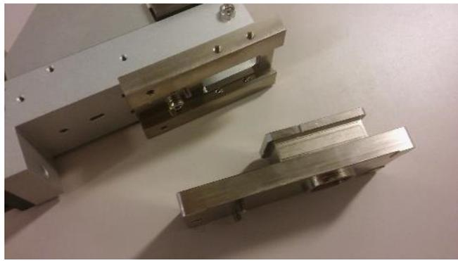
Mount the slid off holder onto the detector using its two hex mounting screws and the pin. Slide the mount and detector back onto the PCC holder.
