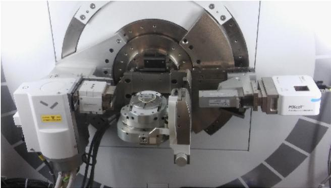
In data collector, go to the instrument tab. Connect the instrument. Select the 5 axis cradle when prompted to select a stage.
