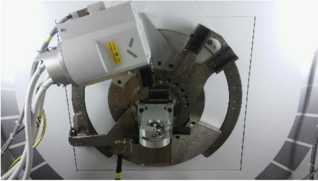
When prompted by the on screen messages remove the reflection transmission spinner stage.
