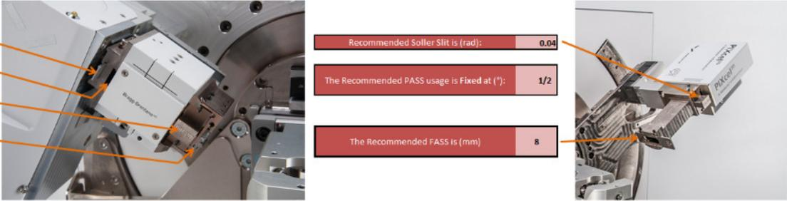
**Do not forget to announce these changes in the configuration in Data Collector. Also, remember to set the PIXcel to Scanning Line (1D) Mode with a full (3.34°) active length in your measurement program.**
