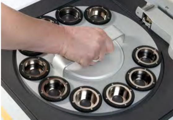
**Figure 6.2** *Put the sample tray onto the sample changer*
