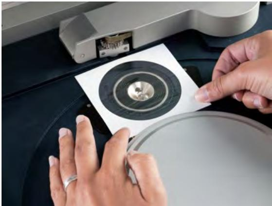
**Figure 6.6 Put the protection foil on top of the measuring position**
