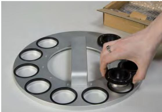
**Figure 4.4** Put the sample holders in the sample tray
