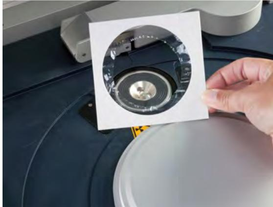
**Figure 6.7** Remove the paper frame
