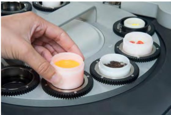
**Figure 6.3** *Put sample cups in the sample holders*
