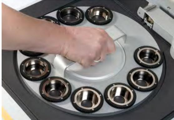
**Figure 4.5 Put the sample tray onto the sample changer**
