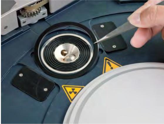
**Figure 6.5 Remove the clamping ring**
