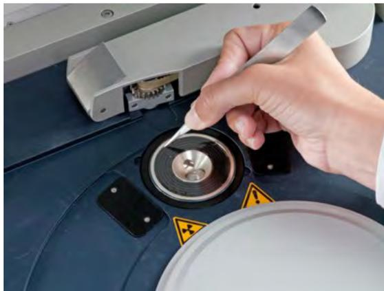
**Figure 6.8** Put small holes in the protection foil
