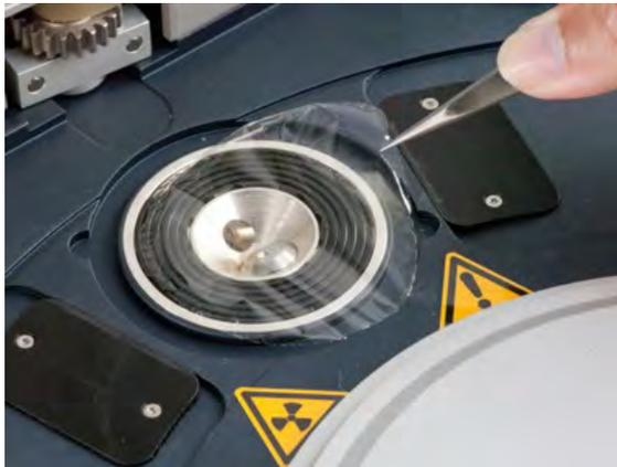
**Figure 6.9** *Remove the protection foil*
