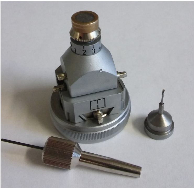
Figure 4, Goniometer head with magnetic snap on mount and adjustment screw
